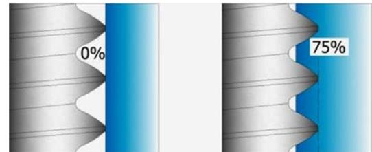
If the nominal diameter of the screw is known, a pilot hole size can be selected for an initial test from the REMINC documents on the basis of the component thickness and resulting thread engagement. Corresponding documents can be downloaded from the REMINC website for TAPTITE 2000® screws.
